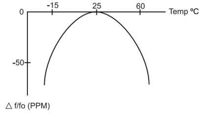
To calculate the frequency stability the parabolic curvature constant (K) is needed. For calculating the stability at 45°C?
