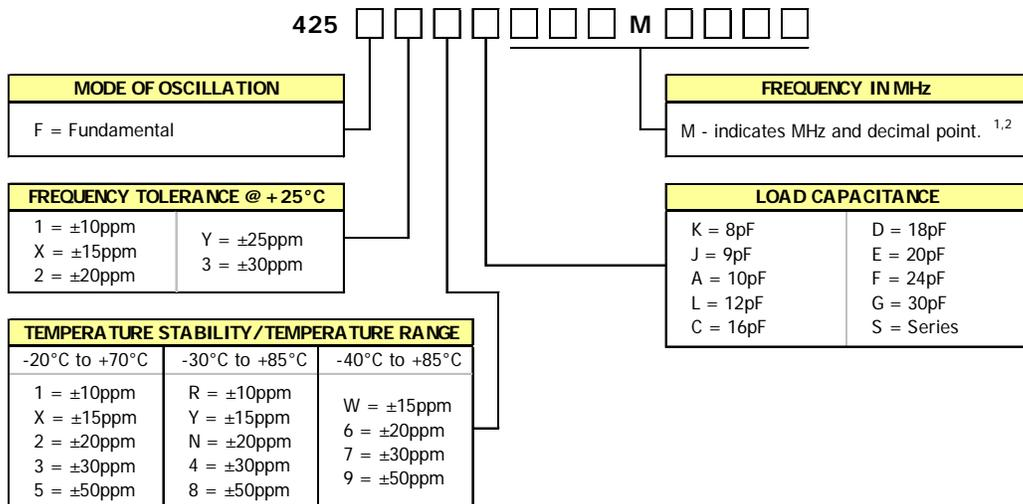
1. Frequency is recorded with 3 leading digits before the 'M' and 4 significant digits after the 'M' [including zeros].
